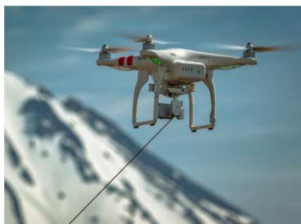
(c) 系留无人机 [12] Tethered UAV (Unmanned Aerial Vehicle)
